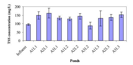
Fig. 4.5. The average values of TSS concentration in the influent and effluent of ABPs, n = 5. The vertical columns represent the average TSS concentration values for the influent and the nine ponds of the pilot plant. The bars represent the standard error at a level of significance  $\rho \le 0.05$ .
