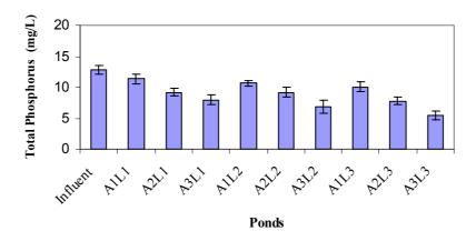
Fig. 4.11. The average values of TP concentration (mg/L) in the influent and effluent of the nine ABPs of the pilot plant of ABPs (represented by columns). The bars represent the values of standard error  $(\pm \sigma/n^{1/2})$ .
