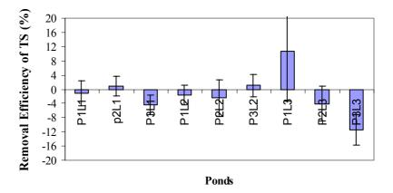
Fig. 4.6. TS removal efficiency from the nine ABPs, n = 9. The columns represent the removal efficiency and the bars represent standard error  $(\pm \sigma/n^{1/2})$ .
