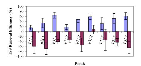
**Fig.4.5.** Average values for the removal efficiencies of TSS in the nine ponds of the two experimental periods. The vertical columns represent the average values TSS removal efficiency. The bars represent the standard error  $(\pm \sigma/n^{1/2})$  at a level of significance  $\rho \le 0.05$ .
