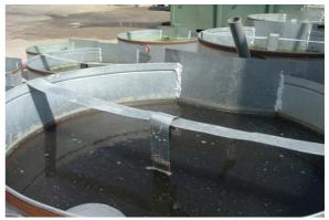
**Photo A.8.** The holder mentioned in A.7, this photo shows particularly the ponds after scavenging the mortared duckweed mat; the whole mat quantity was absolutely removed to prevent decayed duckweed from affecting the readings of different parameters.
