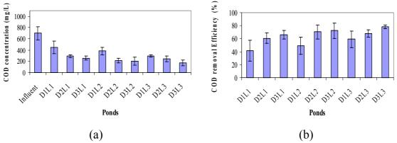
**Fig. 4.7.** Average values of COD concentration at the influent and effluent of DBPs (a) and COD removal efficiency from the nine DBPs (b). The vertical columns represent the average COD concentration values for the influent and the nine ponds of the pilot plant, the bars represent the standard error.
