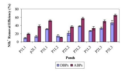
**Fig. 4.15.** Average values for the removal efficiencies (%) of  $NH_4^+$  in the nine ponds of the two experimental periods. The vertical columns represent the average values  $NH_4^+$  removal. The bars represent the standard error  $(\pm \sigma/n^{1/2})$ .
