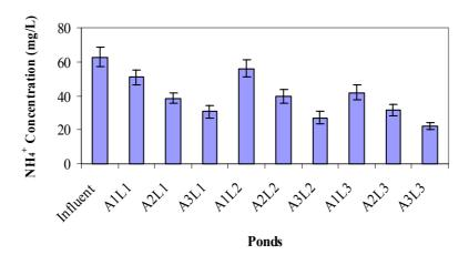
**Fig. 4.14.** The average values of  $NH_4^+$  concentration in the influent and effluent of the nine ABPs (mg/L). The bars represent the standard error  $(\pm \sigma/n^{1/2})$  at a level of significance  $\rho \le 0.05$ .
