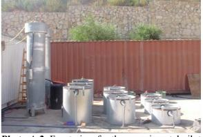
**Photo A.2.** Front view for the experimental pilot plant; the three lines of stabilization ponds and the UASB-septic tanks in AWWTP.
