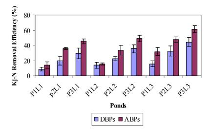
**Fig. 4.18.** Average values for the removal efficiencies (%) of TKN in the nine ponds of the two periods. The vertical bars represent the average values TKN removal. The bars represent the standard error  $(\pm \sigma/n^{1/2})$  at a confidence level.
