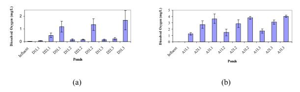
**Fig. 4.2.** DO concentration in DBPs (a) and ABPs (b). The vertical columns represent the average DO concentration in the nine ponds effluent (mg/L); the bars represent the standard error  $(\pm \sigma/n^{1/2})$ . D stands for duckweed and A stands for algae. Note that (D or A)iLj means the i<sup>th</sup> (D or A) pond in the j<sup>th</sup> line (e.g. D<sub>3</sub>L<sub>1</sub>, means the third DBP in the first line).
