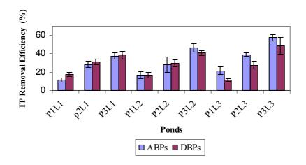
Fig. 4.12. Average values for the removal efficiencies (%) of TP in the nine ponds of the two periods. The vertical columns represent the average values TP removal. The bars represent the standard error  $(\pm \sigma/n^{1/2})$  at a level of significance  $\rho \le 0.05$ .
