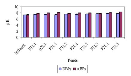
**Fig. 4.3.** Average pH values in DBPs and ABPs. The vertical columns represent the average pH values for the influent and the nine ponds of the pilot plant, the bars represent the standard error  $(\pm \sigma/n^{1/2})$ . n for first and second experimental periods were = 9 and 7, respectively.
