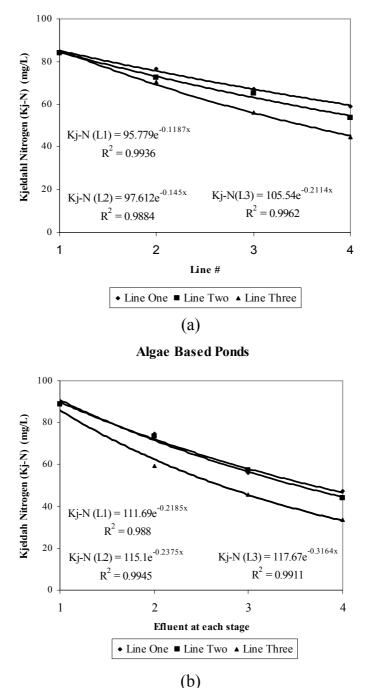
**Fig. A.3.** Removal curve of TKN from the three lines (90, 60, and 30 cm depth ponds) in DBPs (a), and ABPs (b). The figure shows also the best-fit exponential curve and equation for each line with the correlation coefficient between actual points and the curve. Points 1, 2, 3 and 4 (x-axis) represent influent, first, second and third ponds, respectively.
