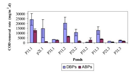
**Fig. 4.9.** Average values for COD removal rates  $(mg/m^2.d)$  for the nine ponds in the two periods. The vertical columns represent the average values COD removal rates. The bars represent the standard error  $(\pm \sigma/n^{1/2})$ .
