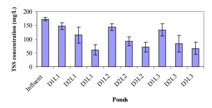
Fig. 4.4. The average values of TSS concentration in the influent and effluent of DBPs, n = 5. The vertical columns represent the average TSS concentration values for the influent and the nine ponds of the pilot plant, the bars represent the standard error  $(\pm \sigma/n^{1/2})$  at a level of significance  $\rho \le 0.05$ .
