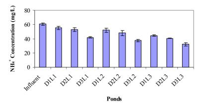
Fig. 4.13, Average values of  $NH_4^+$  concentration in the influent and effluent of the nine ponds of the pilot plant of DBPs (represented by the columns). The bars represent the standard error  $(\pm \sigma/n^{1/2})$ .
