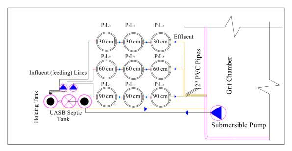
**Fig. 3.1** Schematic diagram for the stabilization ponds based pilot treatment plant; the figure shows the suction location, required pumps, holding tanks, UASB-septic tank, and the three lines of stabilization ponds. The figure shows also each pond with its' corresponding code (which is used later to describe the pond) and depth.
