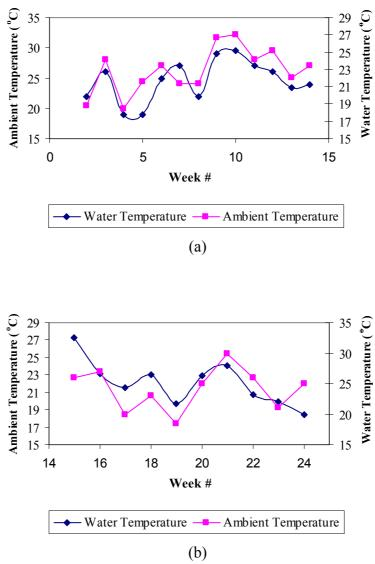
**Fig. 4.1.** Ambient and wastewater temperatures during the DBPs period (a) and ABPs period (b). The number of measurements for the DBPs and ABPs were 13 and 10, respectively.
