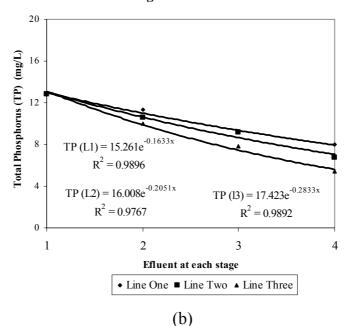
**Fig. A5.** Removal curve of TP for the three lines (90, 60, and 30 cm depth) in DBPs (a), and ABPs (b). The figure shows also the best-fit exponential curve and equation for each line with the correlation coefficient between actual points and the curve. Points 1, 2, 3 and 4 (x-axis) represent influent, first, second and third ponds, respectively.
