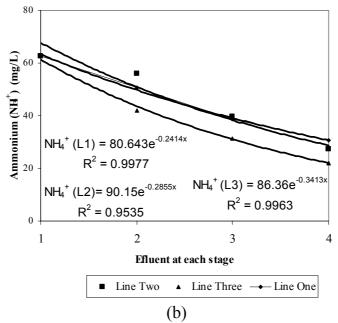
**Fig. A.4.** Removal curve of  $NH_4^+$  from the three lines (90, 60, and 30 cm depth) in DBPs (a), and ABPs (b). The figure shows also the best-fit exponential curve and equation for each line with the correlation coefficient between actual points and the curve. Points 1, 2, 3 and 4 (x-axis) represent influent, first, second and third ponds, respectively.
