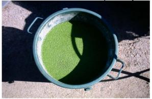
**Photo A.9.** One of duckweed culture, it is a big bucket of dimensions (dia. = 34 cm, L = 40 cm). As mentioned elsewhere, this culture was used as a backup source of duckweed and for testing the duckweed survival in diluted effluent of the UASB-septic tank.
