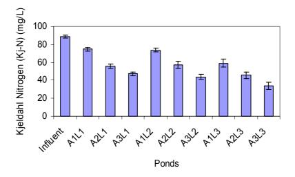
Fig. 4.17. Average values of TKN concentration in the influent and effluent of the nine ABPs. The error bars represent the standard error  $(\pm \sigma/n^{1/2})$  at a level of significance  $\rho \le 0.05$ .
